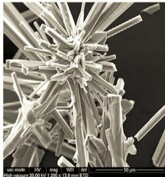
Left: ZnO nanostructures, right: micro-inductor on porous Si substrate. Source: GREMAN Laboratory
